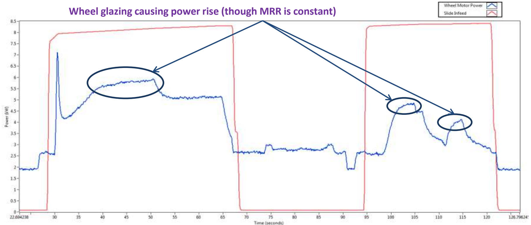
OD profile grinding – work-material with high hardness (62 HRC)
